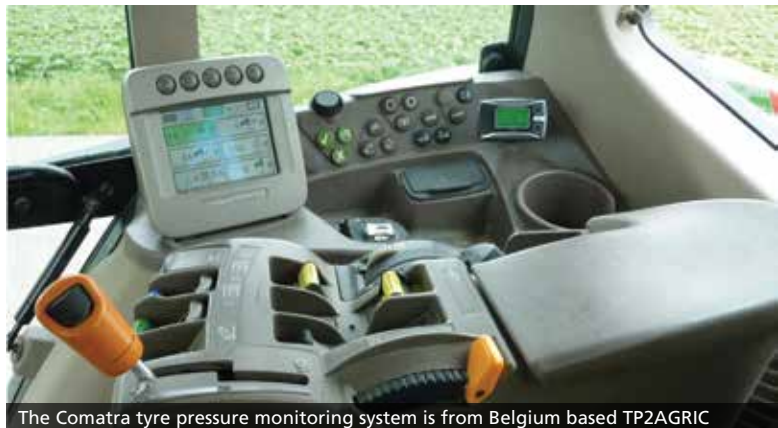
The Comatra tyre pressure monitoring system is from Belgium based TP2AGRIC
