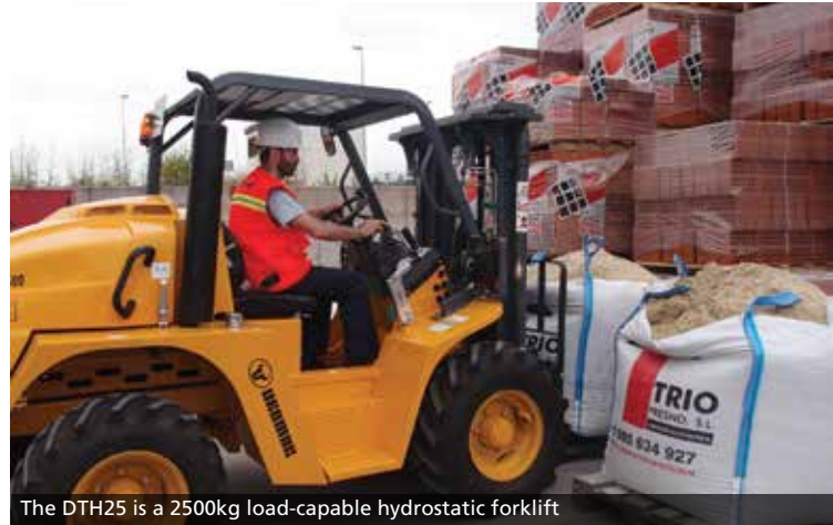
The DTH25 is a 2500kg load-capable hydrostatic forklift
